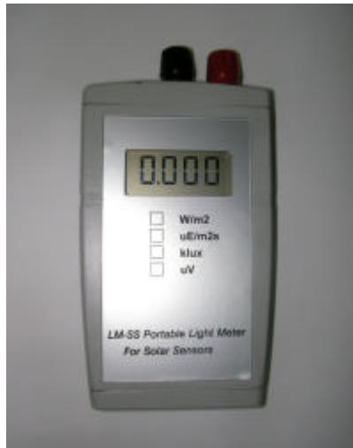
The LM-SS is a low-cost, high-performance sensor readout unit with integrated datalogger.
