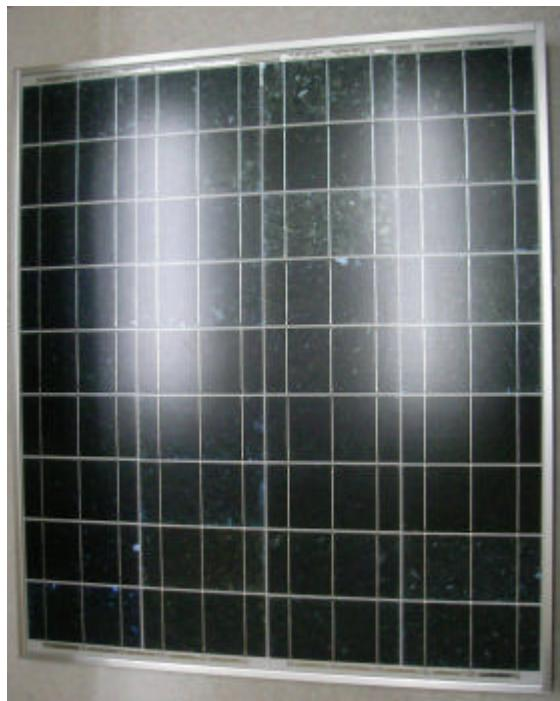
The highly efficient multi crystalline photovoltaic modules are produced by an advance cell processing technology and automated production facilities. These cells are encapsulated between a tempered glass cover and pottant with back sheet to provide efficient protection from the severest environmental conditions. The entire laminate is installed in an anodized aluminum frame to provide structural strength and ease of installation.
