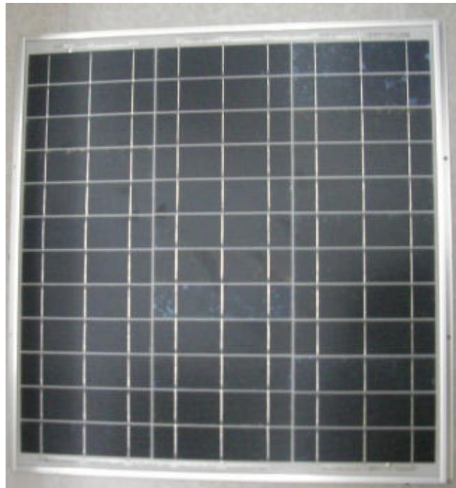
The highly efficient multi crystalline photovoltaic modules are produced by an advance cell processing technology and automated production facilities. These cells are encapsulated between a tempered glass cover and pottant with back sheet to provide efficient protection from the severest environmental conditions. The entire laminate is installed in an anodized aluminum frame to provide structural strength and ease of installation.
