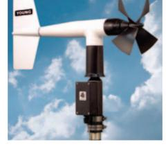
potentiometer housed in a sealed chamber. With a known excitation voltage applied to the potentiometer, the output voltage is directly proportional to vane angle. A mounting orientation ring assures correct realignment of the wind direction reference when the instrument is removed for maintenance.
