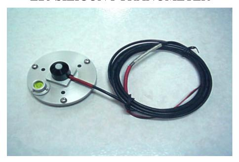
The E20 SILICON PYRANOMETER is designed for routine measurement of solar radiation including following application:
