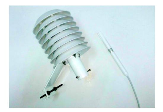
Precision meteorology probes for relative humidity and temperature - HC2S3
